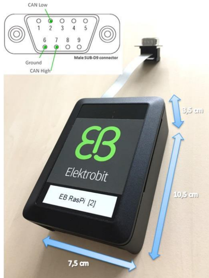
Figure 31: Dimensions of EB robinos Predictor Eval Kit and pin layout of the SUB-D9 connector
